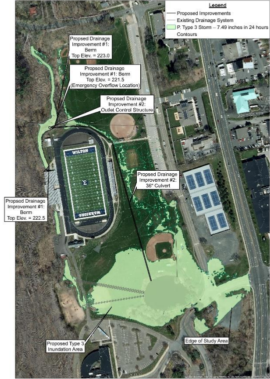
Figure 6: Proposed Type 3 Inundation Area Design Storm: 7.49 inches in 24 hours Wilton, CT
