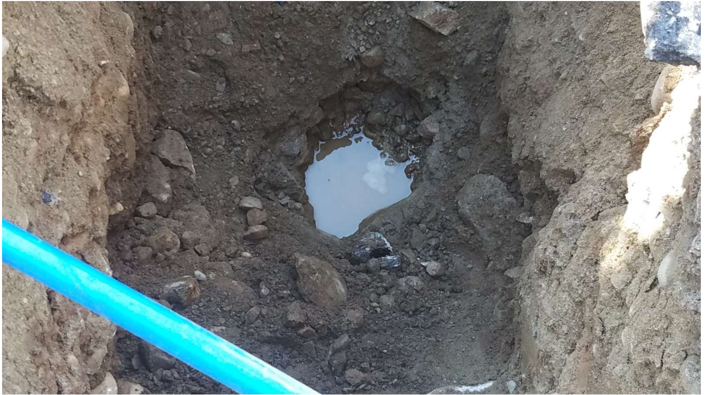
TP-5 percolation test. Top of perc hole is 4' below pavement grade. Water level in hole readily percolated into the ground during the test.
