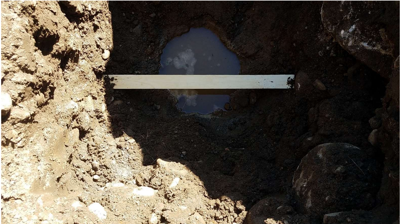
TP-4 percolation test. Top of perc hole is 3' below pavement grade. Water level in hole did not percolate into the soil during the 30 minute +/- duration it was observed.
