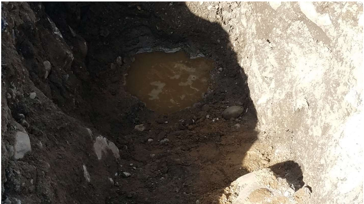
TP-4 percolation test. Top of perc hole is 4' below pavement grade. Water level in hole again did not percolate into the soil during the 30 minute +/- duration it was observed.
