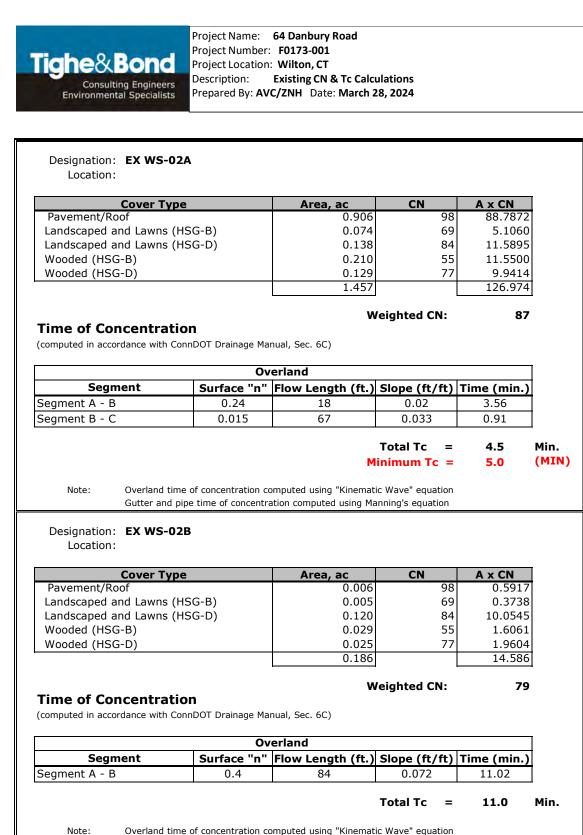
Overland time of concentration computed using "Kinematic Wave" equation Gutter and pipe time of concentration computed using Manning's equation
