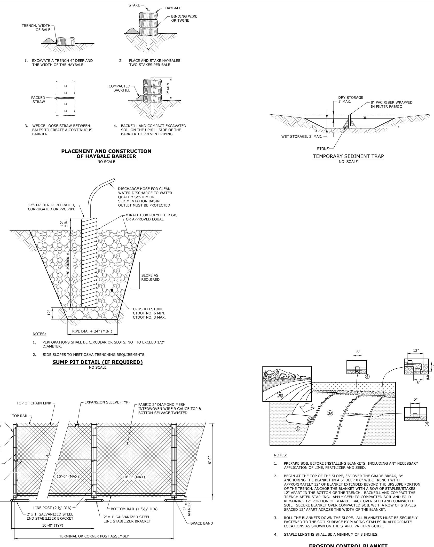
**<u>6' TEMPORARY CHAIN LINK CONSTRUCTION FENCE</u>** NO SCALE
