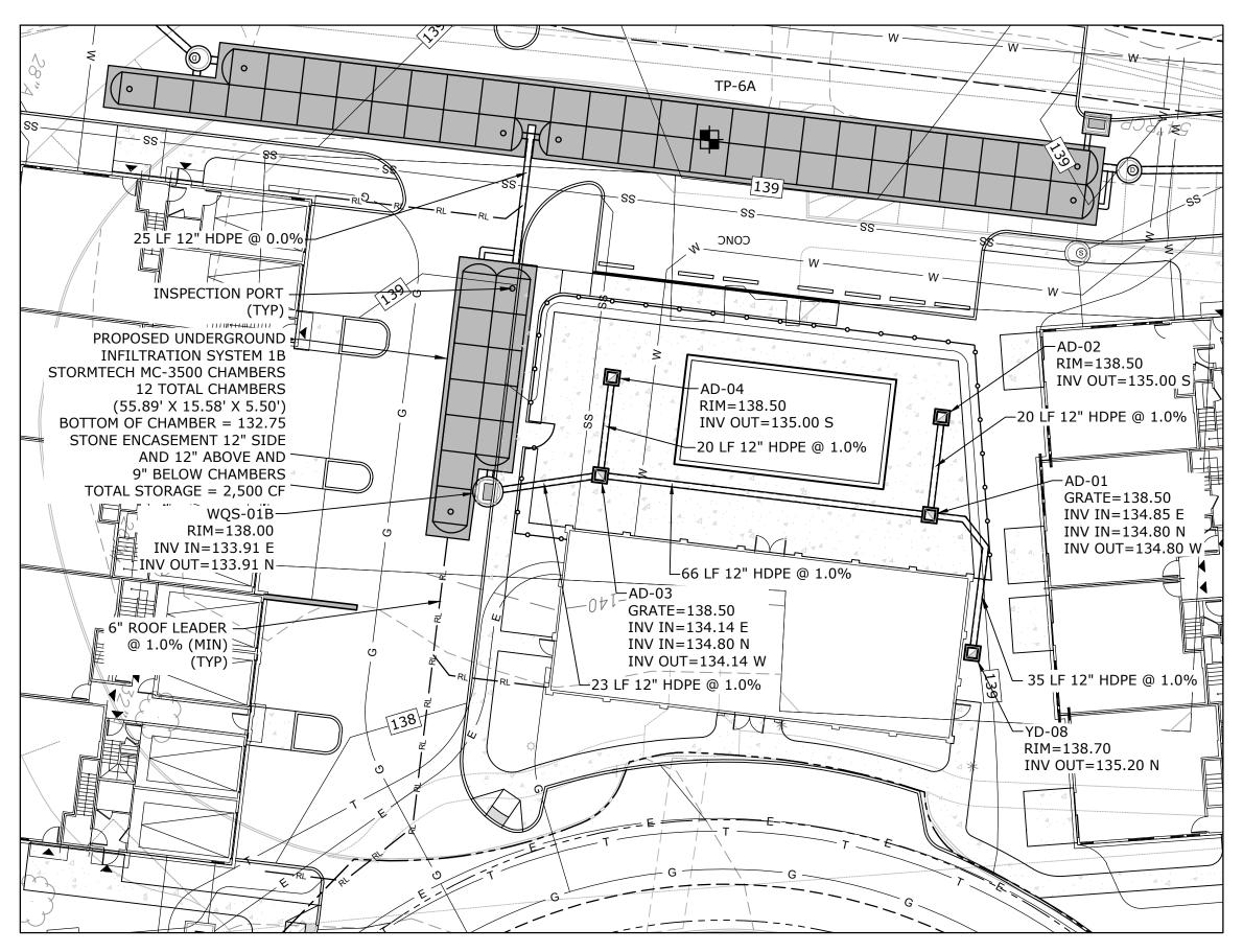
PART PLAN "C" - INFILTRATION SYSTEM 1B SCALE: 1" = 20'
