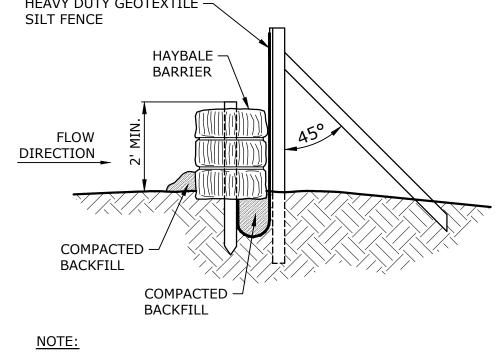
1. BACKFILL AND COMPACT THE EXCAVATED SOIL AS SHOWN ON THE UPHILL SIDE OF THE BARRIER TO PREVENT PIPING.
