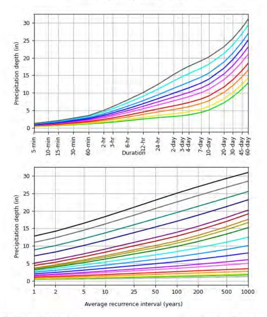
PDS-based depth-duration-frequency (DDF) curves Latitude: 41.1679°, Longitude: -73.4146°
