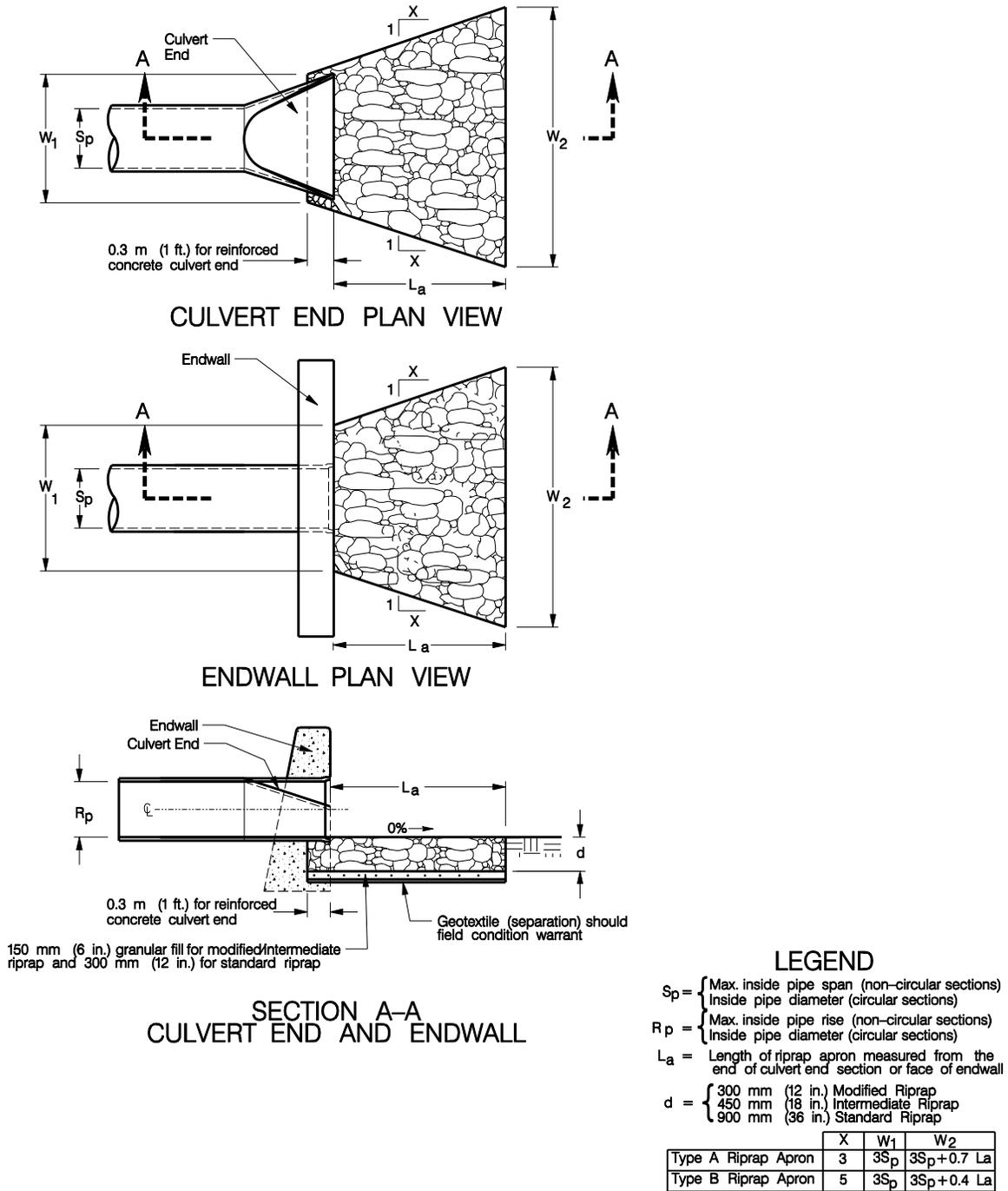
**Figure 11-13 Type A and B Riprap Apron**
