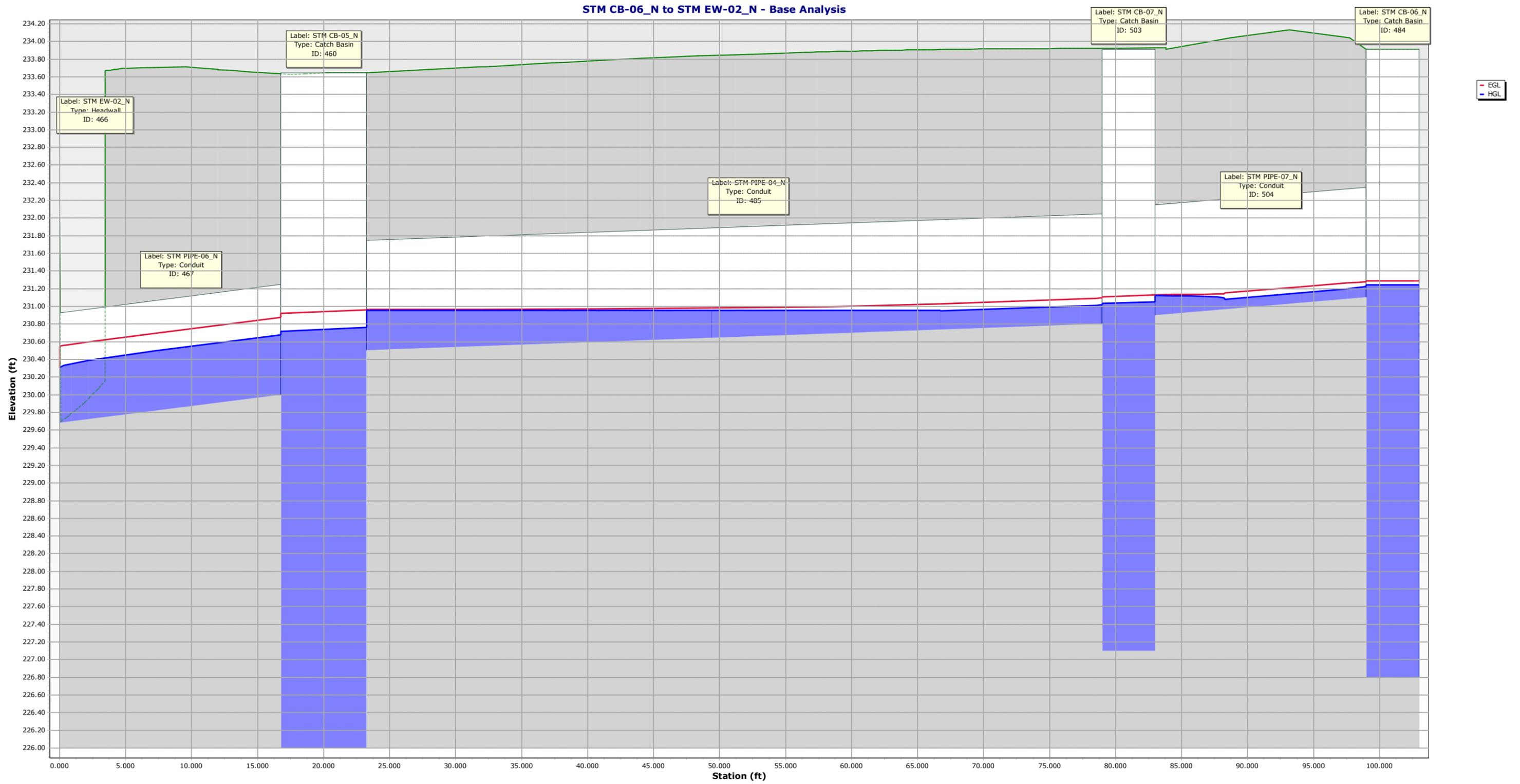
Note: Tailwater Elevation used is 227.50', derived from the FEMA Flood Insurance Study
