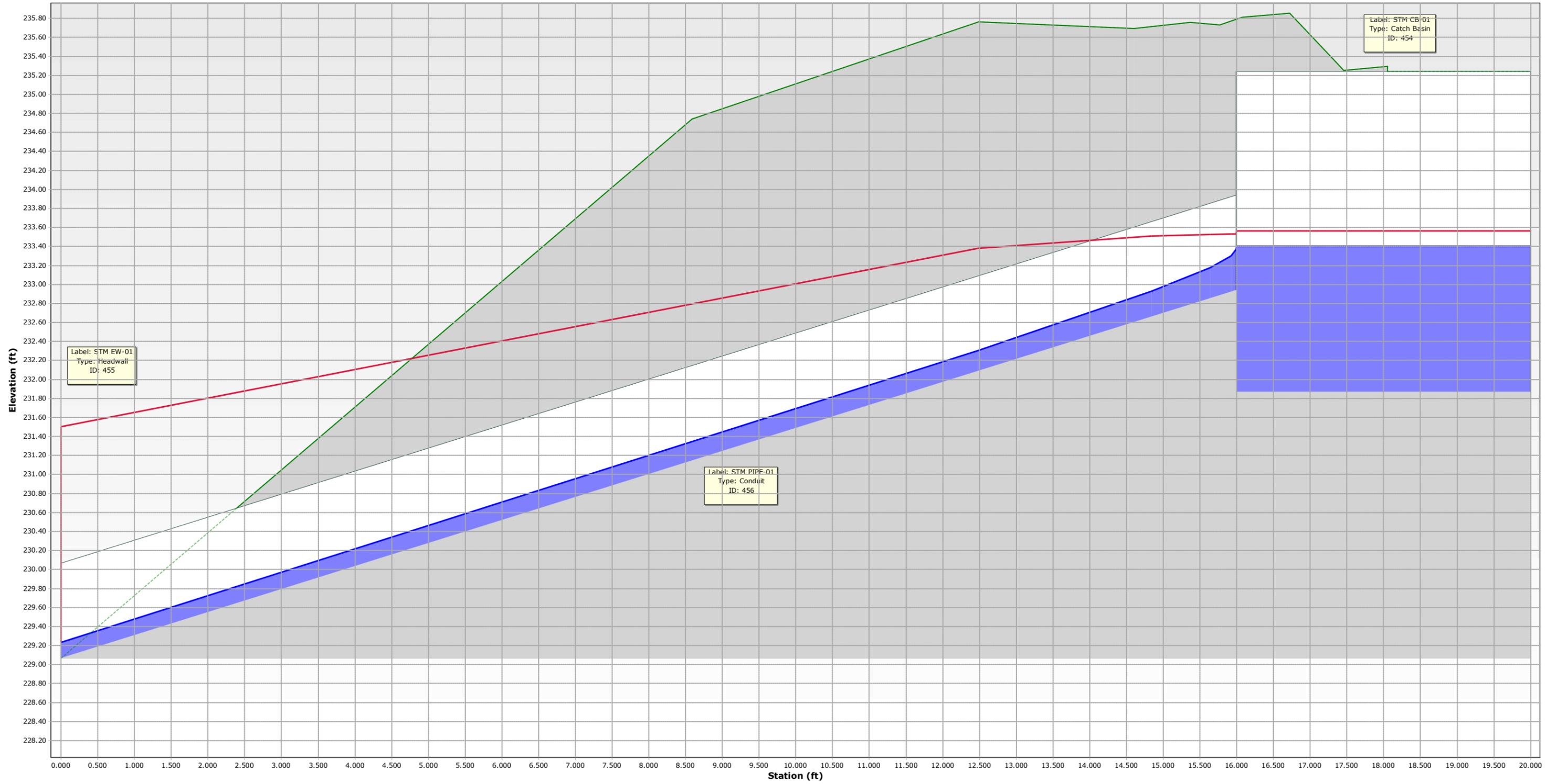
Note: Tailwater Elevation used is 227.50', derived from the FEMA Flood Insurance Study
