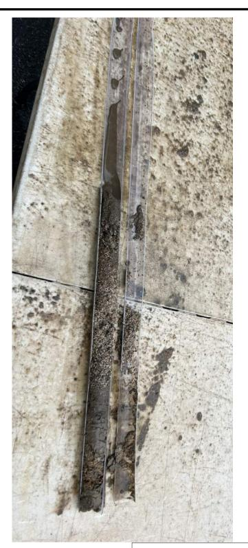
VB- 5 (4.0 to 8.5 FT) <u>Photographer:</u> T. Rezzani Note Filter Sand at top of sample
