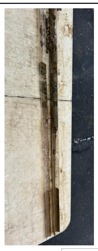
VB- 2 (4.0 to 9.0 FT) <u>Photographer:</u> T. Rezzani Note Filter Sand at top of sample
