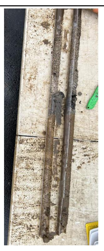
VB- 1 (3.0 to 8.0 FT) <u>Photographer:</u> T. Rezzani Note Filter Sand at top of sample
