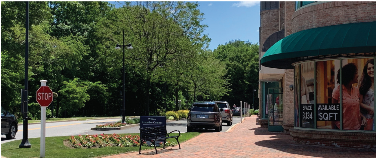
Figure 26 This frontage provides off-street parking in a layby configuration (see Section (A) below). A more pedestrian-friendly configuration removes the separating median and places parallel parking (B) or angled parking (C) next to the roadway. These configurations would allow for a wider and more active sidewalk and create a more people-friendly environment.
