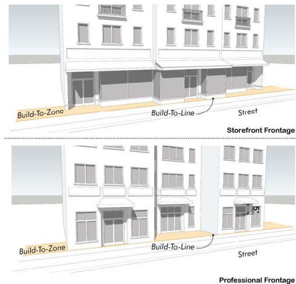
Street frontage diagram showing examples of building placements for WC-1 Storefront Frontage & WC-2 Professional Frontage with a 5-foot Build-To-Zone
