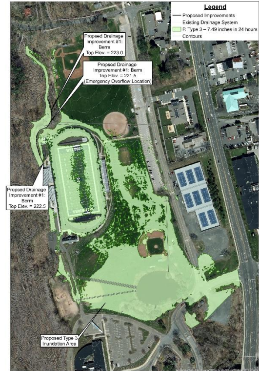
Figure 5: Proposed Type 3 Inundation Area Design Storm: 7.49 inches in 24 hours Wilton, CT
