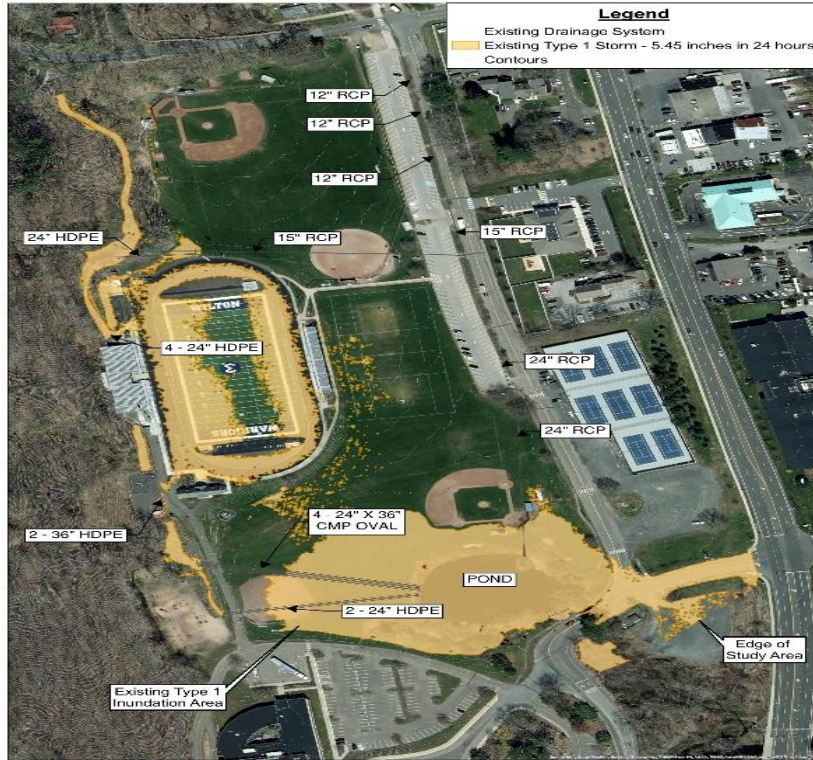
Figure 2: Existing Type I Inundation Area Design Storm: 5.45 inches in 24 hours Wilton, CT
