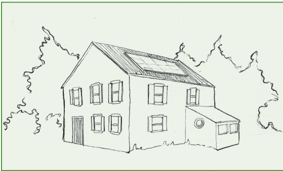
Solar thermal installations sit flush with the roof.
