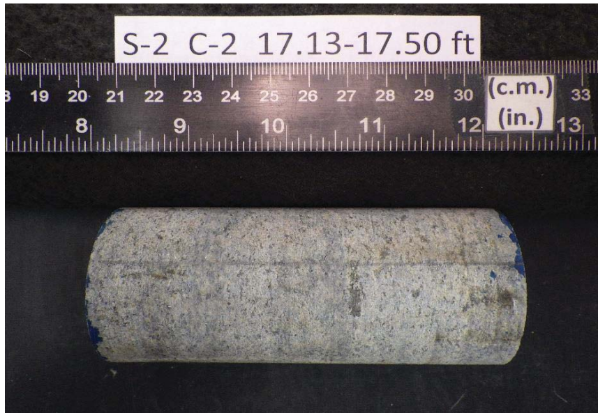
After cutting and grinding
